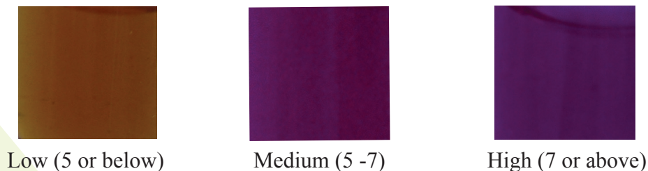
Figure 4. Colour Variation for different levels of soil PH
