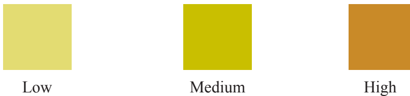
Figure 8. Colour variation for different levels of soil K
