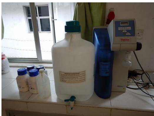
Water Purification System
