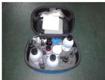
**Figure 1. LaMotte plant sap test Kit**
